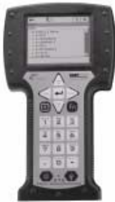
Figure 8. Perform Configuration and Calibration at the Valve or Anywhere on the 4 to 20 mA Loop with the Model 375 Field Communicator
